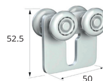
Double axle hanger, 50 x 52.5mm fixing plate, 45kg capacity Code: 20-1086
