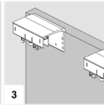
3 Mount the upper roller to outer doors, keeping the adjusting screw facing toward the edges of the door.
