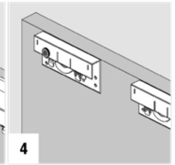
4 Mount the upper roller for inner doors keeping the adjusting screw facing toward the edges of door.
